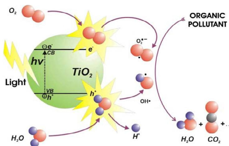
**Fig. 1.** Schematic diagram illustrating the principle of TiO<sub>2</sub> photocatalysis. Reprinted from Ref. [9] under the Creative Commons Attribution License.
