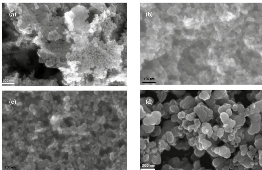
**Fig. 2.** Scanning electron microscope images of the sol-gel prepared TiO<sub>2</sub> powders: (a) sample T-1 synthesized at pH = 4 and annealing temperature (AT) 450 °C, (b) sample T-2 synthesized at pH = 6 and AT 450 °C, (c) sample T-4 synthesized at pH=4 and AT 700 °C, (d) sample T-5 synthesized at pH = 4 and AT 850 °C.
